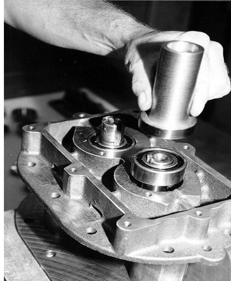
Figure A3. Tapping Bearings into End Plates
