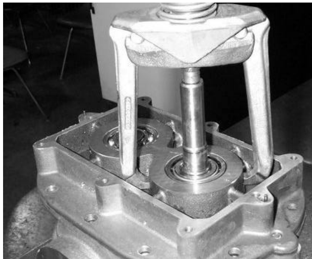
Figure 5. Pulling Drive End Plate
