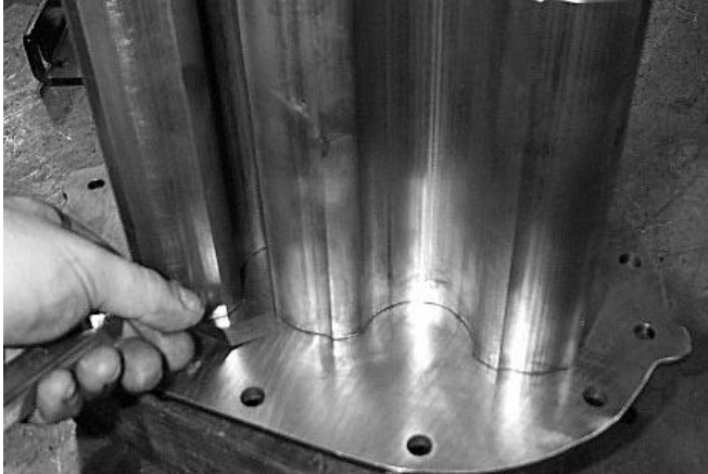
Figure A4. Checking Gear End Clearances
